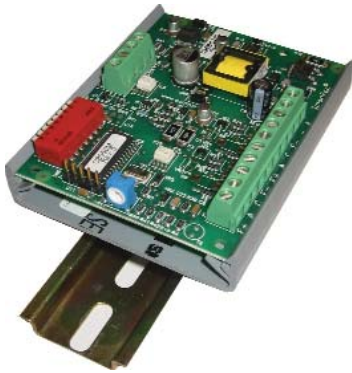
CRI #036BCT00-F with DIN350-F DIN rail kit (sold separately).
